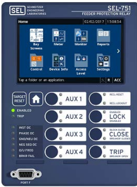
Five-inch, Color Touchscreen Display Model With Eight Pushbuttons
